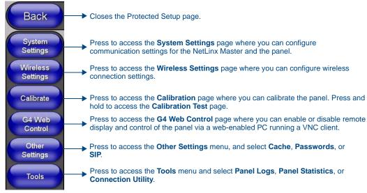
FIG. 50 Protected Setup Navigation Buttons (MVP-8400)
